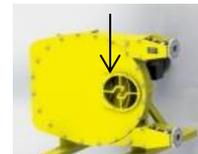
2. Check the state of the cover seal and replace it if necessary.
