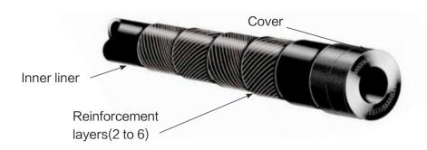
We only work with high quality compounded rubbers, reinforced with 2 to 6 individual layers of braided polyamide and with an outer layer made to strict tolerances to ensure perfect compression.
