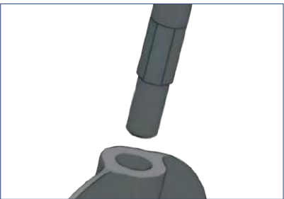
The pinless valve stem features a hexagonal design
